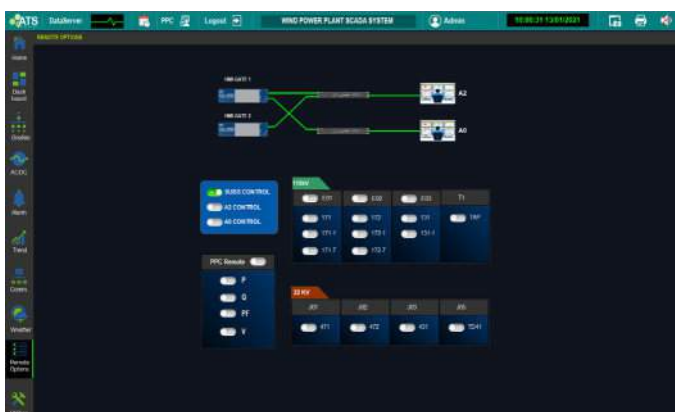
Figure 18. SCADA Channel Status and Control
