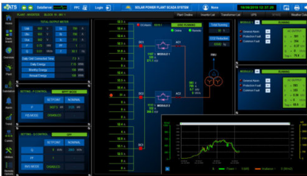
Figure 12. PV Inverter Data Monitoring and Control
