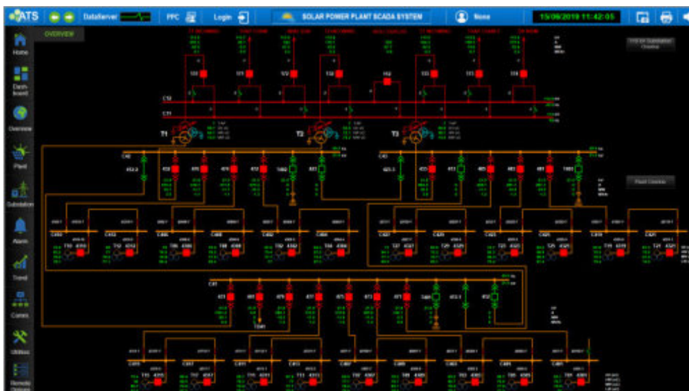
Figure 10. PV Power Plant Single Line Diagram
